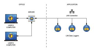
When used as part of a Tinytag Connect system, the logger transmits data to a Windows service that runs the system, called the Connect Gateway. This data is then viewed, and loggers configured, using the Connect version of Tinytag Explorer.
