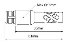
A **PBRF-8002** temperature and relative humidity probe and **CAB-0034** sensor extension cable are provided with the data logger.
