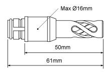
2 x PBRF-8002 temperature and relative humidity probes and CAB-0034 sensor extension cables are provided with the data logger.
