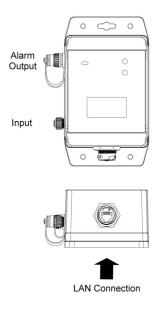
This logger can be used with a CAB-3239 Tinytag Voltage/XP Input Lead (supplied) or an ACS-9703 5-Pin Plug.
