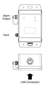
This logger can be used with a CAB-3246 Tinytag Current/Millivolt/Count Input Lead (supplied) or an ACS-9700 2-Pin Plug.
