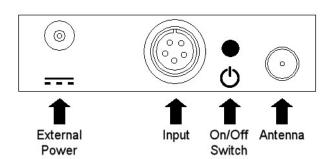
This logger can be used with a CAB-3239 Tinytag Voltage/XP Input Lead (supplied) or an ACS-9703 5-Pin Plug.
