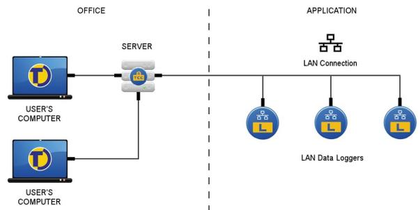
When used as part of a Tinytag Connect system, the logger transmits data to a Windows service that runs the system, called the Connect Gateway. This data is then viewed, and loggers configured, using the Connect version of Tinytag Explorer.
