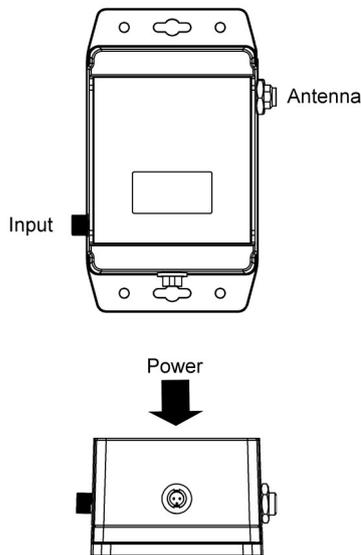
This logger can be used with a CAB-3246 Tinytag Current/Millivolt/Count Input Lead (supplied) or an ACS-9700 2-Pin Plug.
