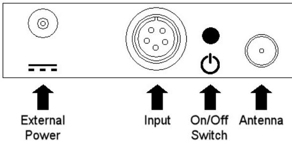
This logger can be used with a CAB-3239 Tinytag Voltage/XP Input Lead (supplied) or an ACS-9703 5-Pin Plug.
