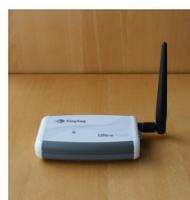
The logger can also be positioned on a non-conductive flat surface, such as a desk or a shelf, with its antenna positioned vertically, with no loss of performance.
